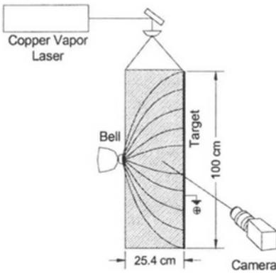
**Fig. 5** The visualization set up of the spray
