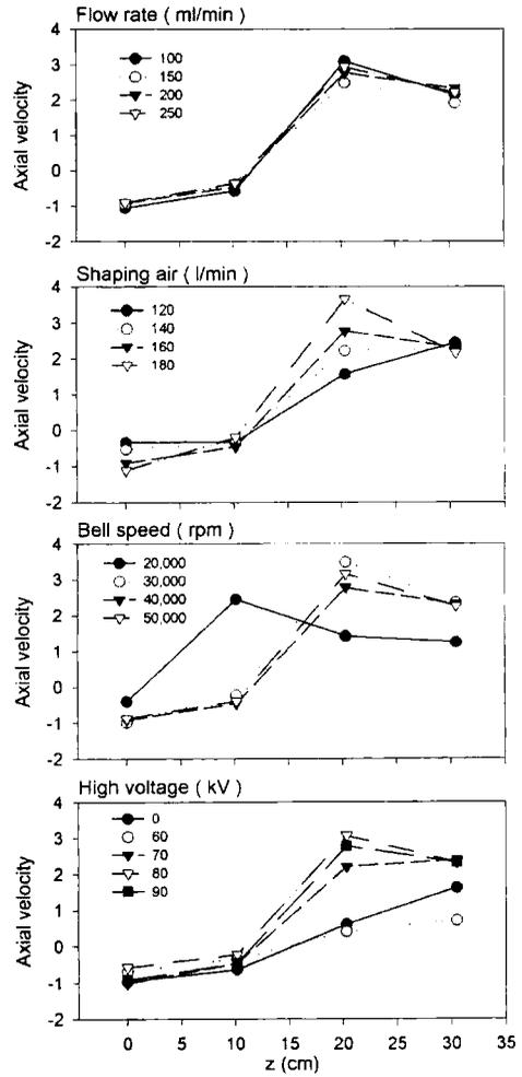
Fig. 18 The effects of the bell operation parameters on the axial velocity at 7.62 cm from the target
