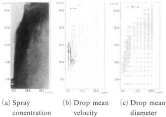
**Fig. 8** The spray structure at the condition of 50 ml/min liquid flow rate 150 l/min, shaping air, 30 k rpm bell speed, and 90 kV voltage setting
