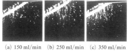
**Fig. 10** Microscopic visualization on the liquid flow rate at the bell speed=20 k rpm (Magnification=100 x)
