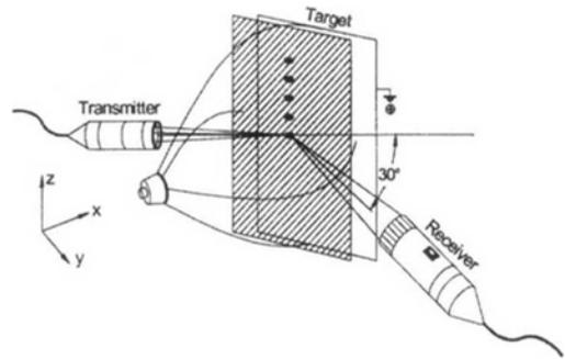
**Fig. 6** The drop size measurement set up by the phase Doppler particle analyzer
