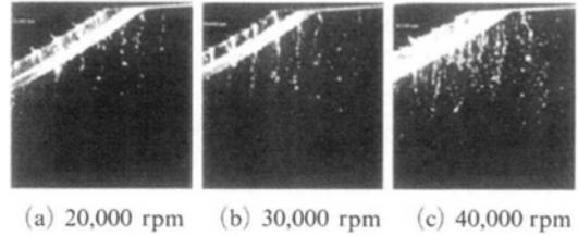
**Fig. 9** Microscopic visualization on the bell speed at the liquid flow rate=50 ml/min (Magnification=100x)
