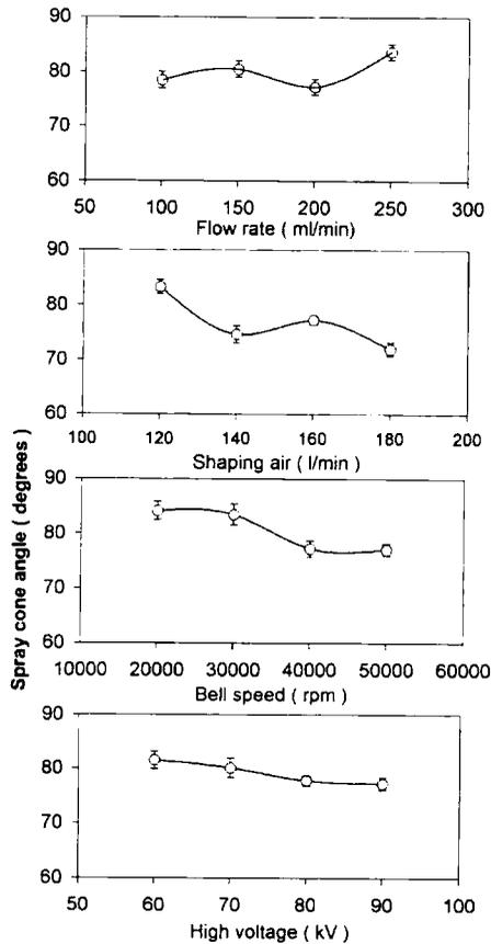
Fig. 15 Sensitivity of the bell operation parameter on the spray cone angle
