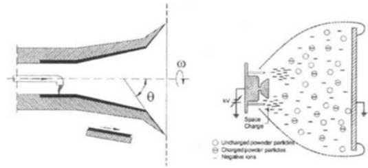
**Fig. 1** The principle of the rotating cup atomization and the electrostatic spray
